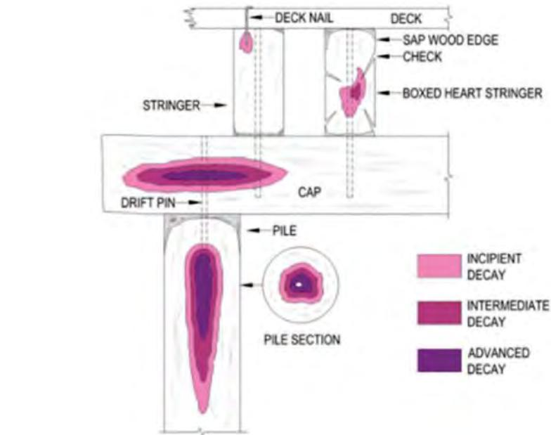
Shows the level of decay that occurs in timber due to the use of vertical fasteners. Vertical fasteners increase the rate of decay in timber as they allow moisture to travel down the fastener into the heartwood of the cap, stringers, corbels and piles, therefore increasing the moisture content in the middle of these elements.
